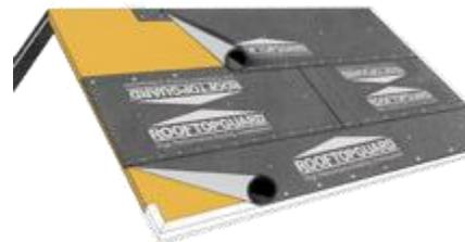
Except in cases where Clay or Concrete tiles are to be installed. In those cases where the slope is 2 ½ :12 up to 4:12, the underlayment must be horizontally lapped a minimum of 30" [763 mm] to the center line of the underlying course to form a double layer with 6" [152 mm] vertical laps.
